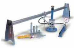
PLATE BEARING TEST
